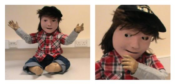
Figure 3.7: KASPAR 1b, the second and improved model of minimally-expressive robots built by the University of Hertfordshire [Robins et al., 2010]
