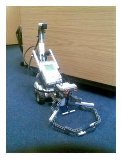
Figure 3.2: The NXT robot used in my first experiment. Its design was inspired by the Tribot configuration
