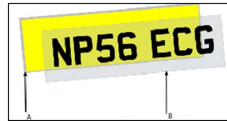
(b) Thin Film Based Number Plate Construction. A is a self adhesive retroreflective film attached to rigid plastic sheet. B indicates Registration marks printed on rest of the film
