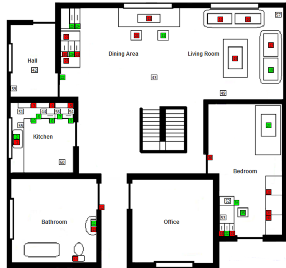
Figure 1: UH Robot House map showing the location of sensors (identified by numbers) and their states with green colour representing the sensor in open/on/free state, red colour representing the sensor in closed/off/occupied state and transparent representing the sensor in a not activated/unknown state.
