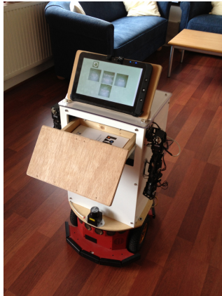
Figure 4: The Replacement Sunflower Robot (SF3) extends its tray and offers to carry an object for the user.
