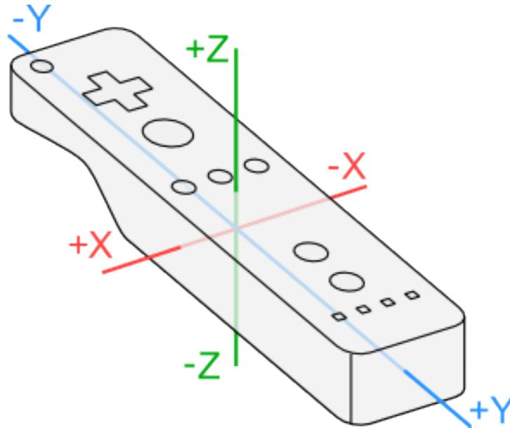
Figure 4.6: The axes of each Wiimote according to their accelerometers. “Pitch” or “Tilt” was considered a rotation about the red X-axis, and “roll” was considered a rotation about the blue Y-axis (from <http://wiibrew.org/wiki/Wiimote>).
