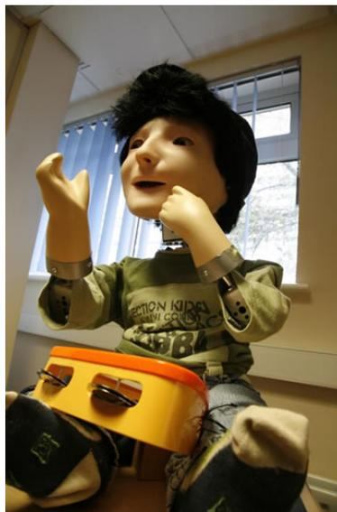
Figure 3.6: KASPAR 1a, the first model of minimally-expressive robots built by the University of Hertfordshire [Dautenhahn et al., 2009]
