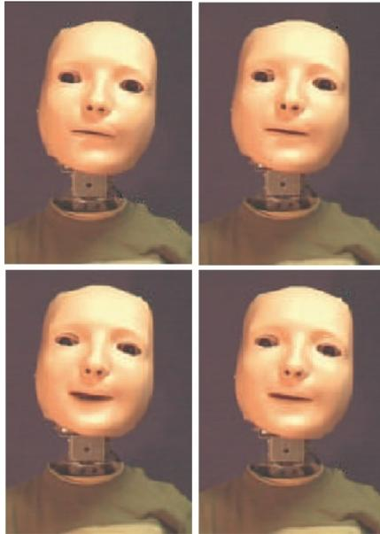
Figure 3.5: Four different facial expressions that KASPAR can make. Clockwise from the top left, they are: neutral, small, medium, and large smiles [Blow et al., 2006].
