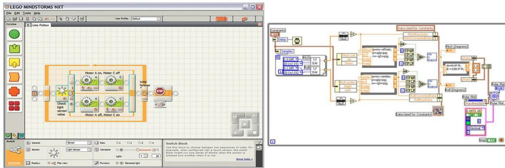
Figure 3.3: Screenshots of the programming languages used on the NXT robots. **Left:** The NXT-G graphical programming environment which the children used (from <http://find.botmag.com/100701>). **Right:** The LabVIEW G programming language which I used to create custom NXT-G programming blocks for the children to use [Litwhiler and Lovell, 2004].
