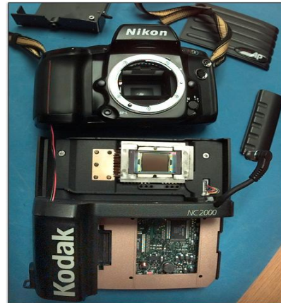
Fig 2.3 Exploded view of a standard digital SLR camera
