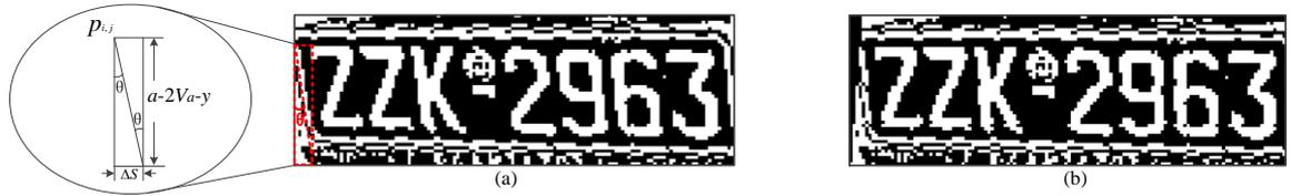
Figure 6-7: (a) NP image before vertical correction. (b) NP image after vertical correction
