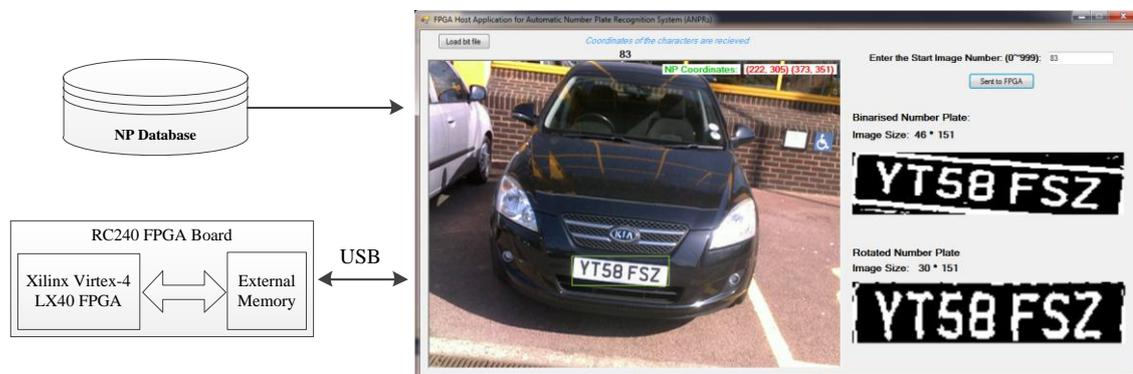
Figure 6-16: Host application for NP binarisation and adjustment
