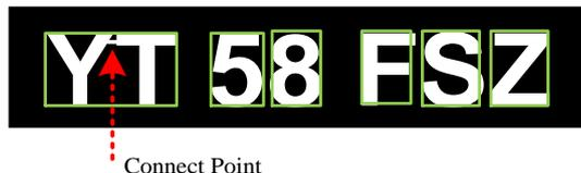
Figure 2-6: A failed example of CS when using the CCA algorithm only
