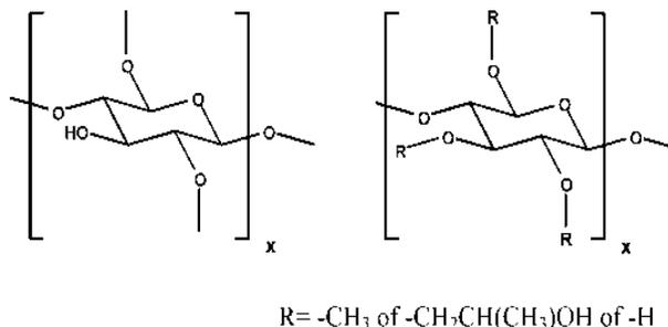
**Figure 6.** Chemical structure of methyl cellulose (left) and (hydroxypropyl)methyl cellulose (right)<sup>[14]</sup>
