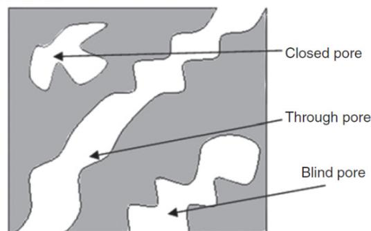
Figure 2: Different pore configurations<sup>[73]</sup>
