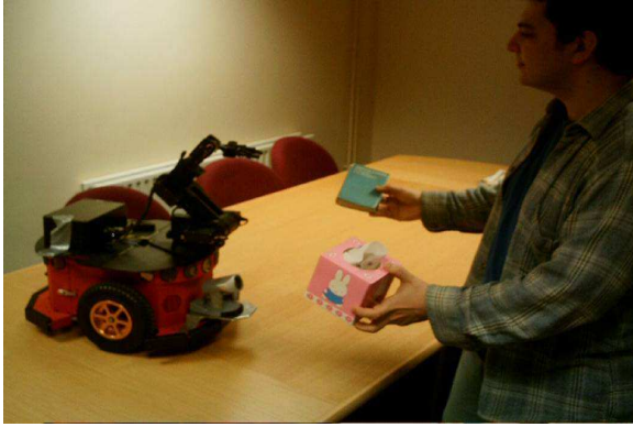
Fig. 1. The environment showing the Pioneer robot with pan/tilt camera and 5-DOF arm.
