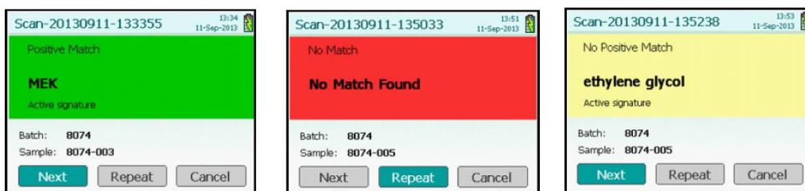
**Figure 1. 4:** A screenshot of the ‘actionable’ results obtained with Truscan™ GP using the PVAL algorithm. Sample responses include ‘positive match’ (left), ‘no match found’ (middle) and ‘no positive match’ (right) (© 2015 Thermo-Fisher Scientific Inc. All rights reserved. All trademarks are the property of Thermo-Fisher Scientific Inc. and its subsidiaries).
