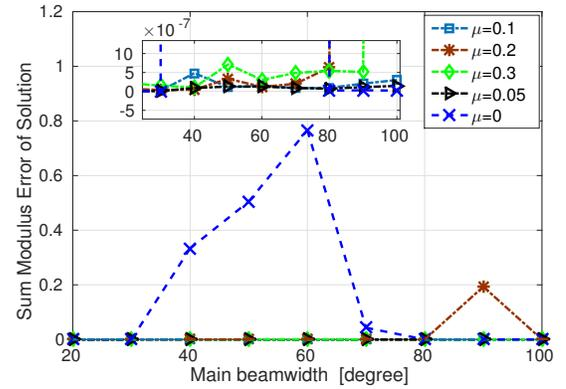
Fig. 4: Sum error  $\|\delta\|_2$  w.r.t. main beamwidth.
