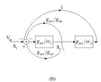
Fig. 5. Tow-Thomas filter to bandpass oscillator conversion (a) using two OTAs and MOS switches and (b) topology (Fig. 4(a)).
