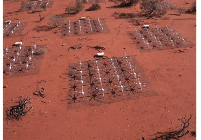
**Figure 1.** Examples of the MWA’s aperture array antenna ‘tiles’, each comprised of a  $4 \times 4$  grid of individual bow-tie dipoles (Image credit: MWA Project, Curtin University).
