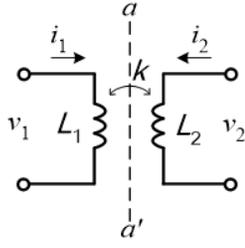
Fig. 5. A two-port network comprising two inductors including mutual coupling.
