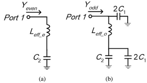
Fig. 4. Even- and odd-mode analysis of the LC-equivalent circuit: (a) even-mode, (b) odd-mode.
