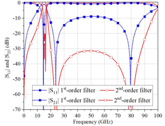
Fig. 12. S-parameters of the designed BPFs using inverting-coupled structure.
