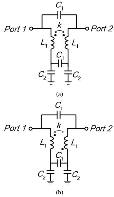
Fig. 3. Simplified LC-equivalent circuit models for the resonators in Fig. 2: (a) with non-inverting coupled one; (b) with inverting coupled one.
