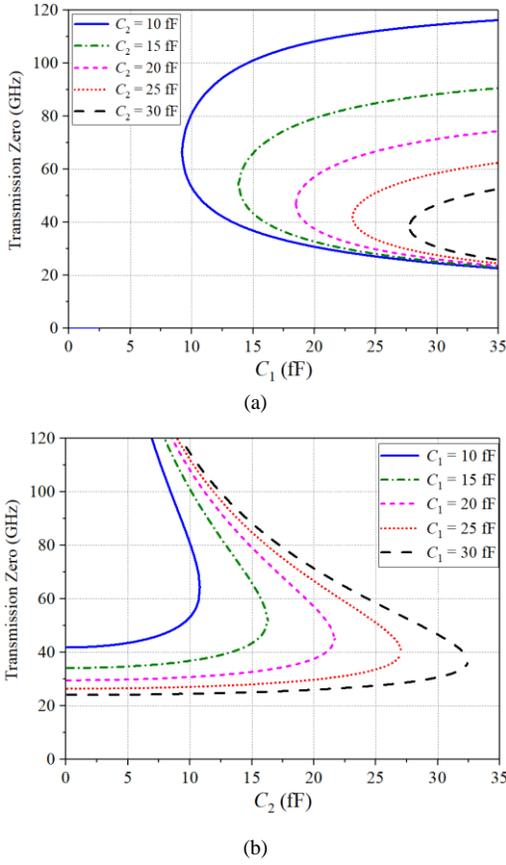
Fig. 10. The values of transmission zeros (a) varying against  $C_1$  when  $C_2$  is fixed; (b) varying against  $C_2$  when  $C_1$  is fixed.
