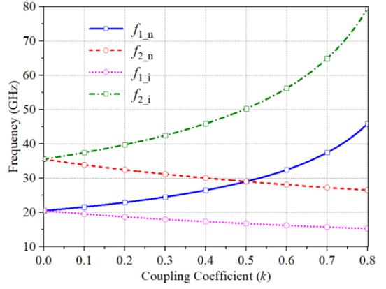
Fig. 7. Resonant mode distribution of  $f_{1n}$ ,  $f_{2n}$ ,  $f_{1i}$  and  $f_{2i}$  against  $k$ . Related parameter values are:  $L_1 = 1000$  pH,  $C_1 = 20$  fF,  $C_2 = 20$  fF.
