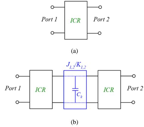
Fig. 11. Configuration of (a) a conventional 1<sup>st</sup>-order BPF; (b) a conventional 2<sup>nd</sup>-order BPF. Note: ICR stands for inverting-coupled resonator.
