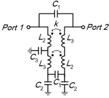
Fig. 15. Simplified LC-equivalent circuit of the modified inverting-coupled resonator.
