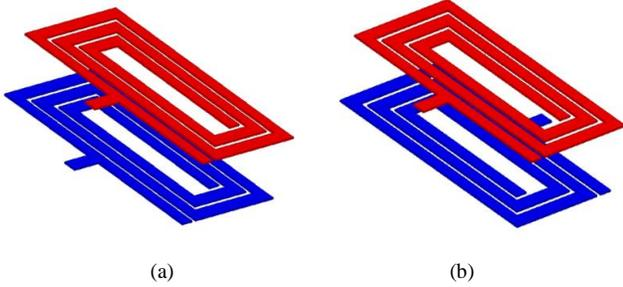
Fig. 2. Two types of resonators using coupled inductors: (a) non-inverting coupled type; (b) inverting coupled type.
