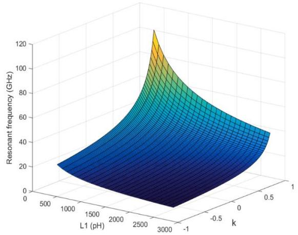
Fig. 9. 3D mapping of resonant frequency  $f_1$  against  $k$  and  $L_1$ .
