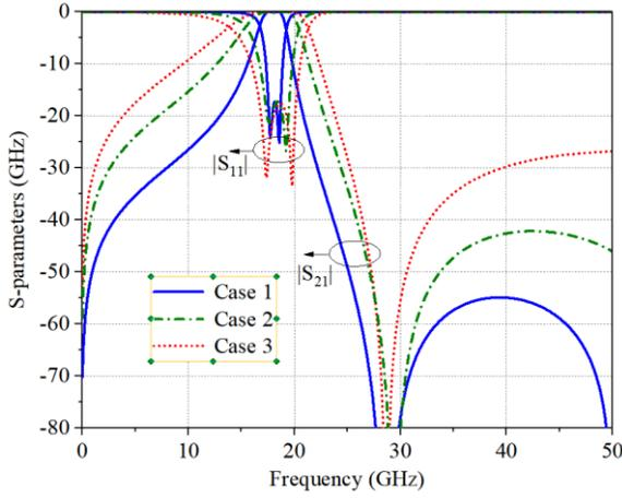
Fig. 17. S-parameters of three 2<sup>nd</sup>-order BPFs using MICR with different bandwidths.
