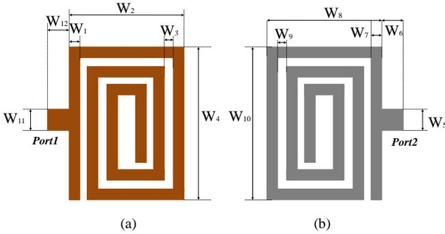
Fig. 14. Layout of the 1<sup>st</sup>-order BPF: (a) upper layer spiral, and (b) lower layer spiral. Note:  $W_1 = 6 \mu\text{m}$ ,  $W_2 = 74 \mu\text{m}$ ,  $W_3 = 4 \mu\text{m}$ ,  $W_4 = 190 \mu\text{m}$ ,  $W_5 = 12 \mu\text{m}$ ,  $W_6 = 12 \mu\text{m}$ ,  $W_7 = 6 \mu\text{m}$ ,  $W_8 = 74 \mu\text{m}$ ,  $W_9 = 4 \mu\text{m}$ ,  $W_{10} = 190 \mu\text{m}$ ,  $W_{11} = 12 \mu\text{m}$ , and  $W_{12} = 12 \mu\text{m}$ .
