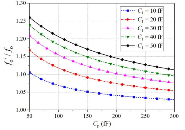
Fig. 18. The frequency ratio of  $f'_o/f_o$  against  $C_p$  when  $C_1$  varies from 10 fF to 50 fF.
