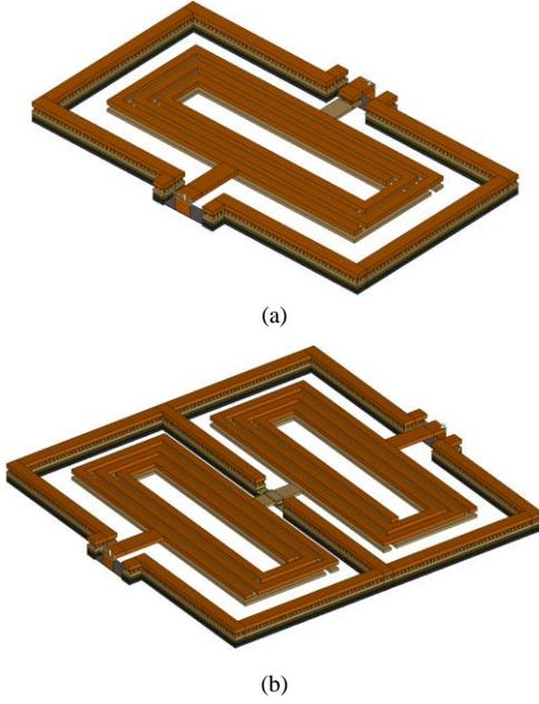
Fig. 13. 3-D views of the designed BPFs, (a) 1<sup>st</sup>-order one, (b) 2<sup>nd</sup>-order one.
