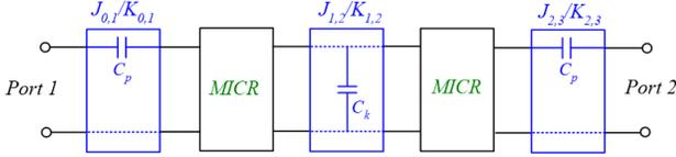
Fig. 16. Configuration of a 2<sup>nd</sup>-order BPF with controllable external  $Q$ -factor.
