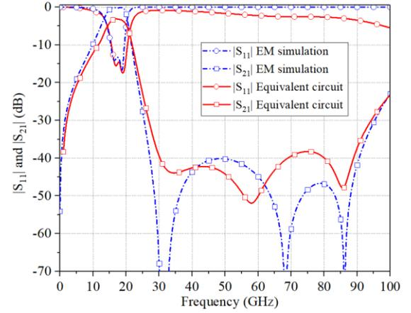
Fig. 20. Comparisons between the S-parameters of the modified 2<sup>nd</sup>-order BPF obtained from EM simulation and simplified circuit model.
