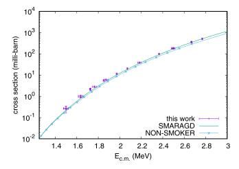
**Figure 4.** Comparison of the experimental  $^{96}$ Zr(p,n) $^{96}$ Nb cross sections with theoretical values obtained with the default settings of the NON-SMOKER and SMARAGD codes.
