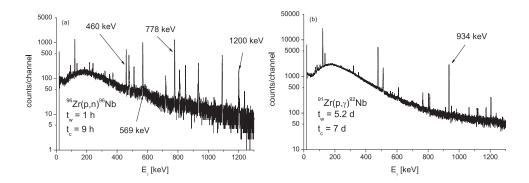
**Figure 2.** Typical  $\gamma$ -spectra measured 1 hour (left panel) and 5.2 days (right panel) after irradiation for 9 hours and 7 days, respectively. The left spectrum was used for the  $^{96}$ Zr(p,n) $^{96}$ Nb cross section evaluation while the right one for the  $^{91}$ Zr(p, $\gamma$ ) $^{92m}$ Nb reaction. The  $\gamma$ -peaks used for the analysis are indicated.
