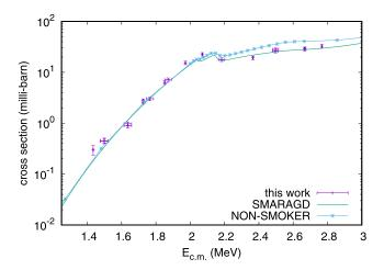
**Figure 3.** Comparison of the experimental  $^{91}Zr(p,\gamma)^{92m}Nb$  cross sections with theoretical values obtained with the default settings of the NON-SMOKER and SMARAGD codes for  $^{91}Zr(p,\gamma)^{92}Nb$ . As detailed in the text, the theoretical curves are for the total, while the experimental data for the isomeric cross sections.
