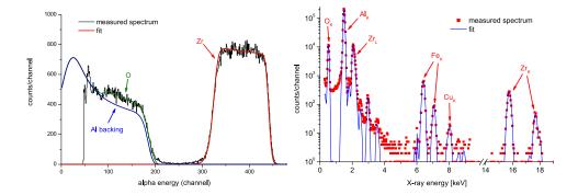
**Figure 1.** RBS (left panel) and PIXE (right panel) spectra measured for the target thickness determination. Fits of the measured data are also shown and the various components of the targets are indicated.
