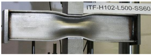
Figure 4 Experimental setup for ITF specimen tests.
