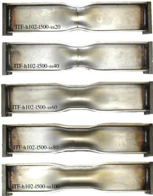
Figure 5 Failure modes of ITF-I102 specimens under internal two-flange (ITF) loading [9].
