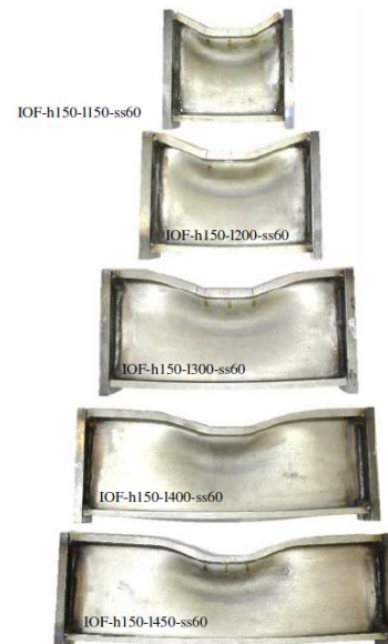
Figure 3 Failure modes of IOF-I150 under internal one-flange (IOF) loading [9].
