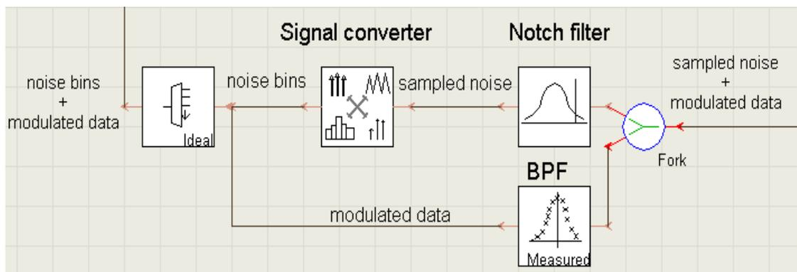
**Figure 5-11** Sampled noise to noise bins conversion model
