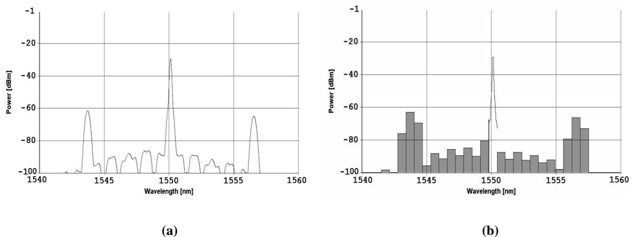
**Figure 5-13 Representation of upstream transmission prior detection in the OLT (a) samples (b) noise bins**
