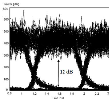
Figure 5-4 Extinction ratio of RSOA transmitted signal
