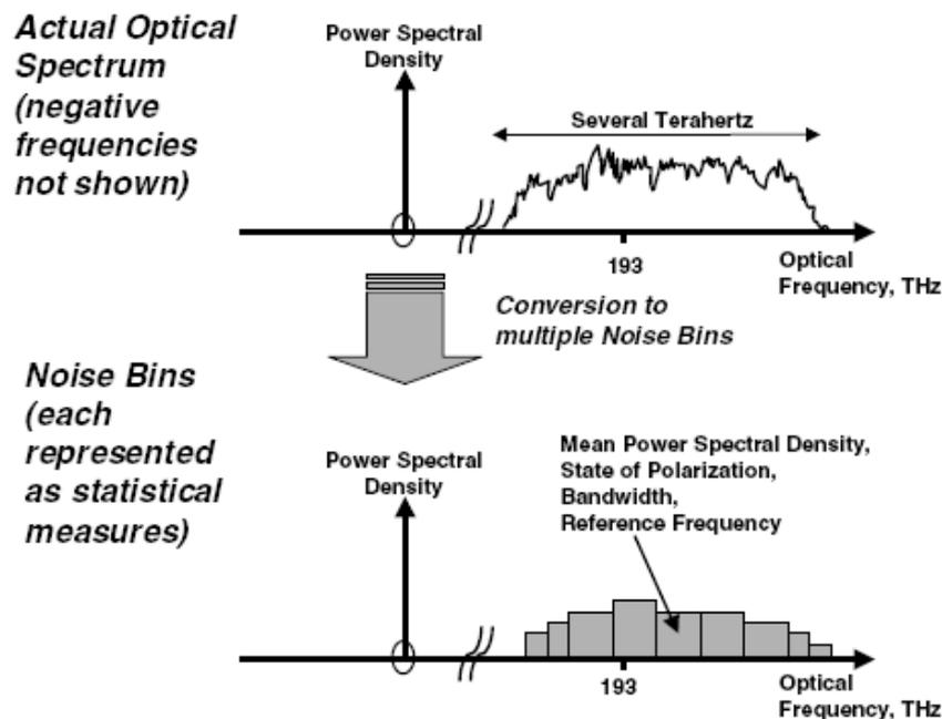
Figure 5-10 Representation of wide-band noise with noise bins [17]
