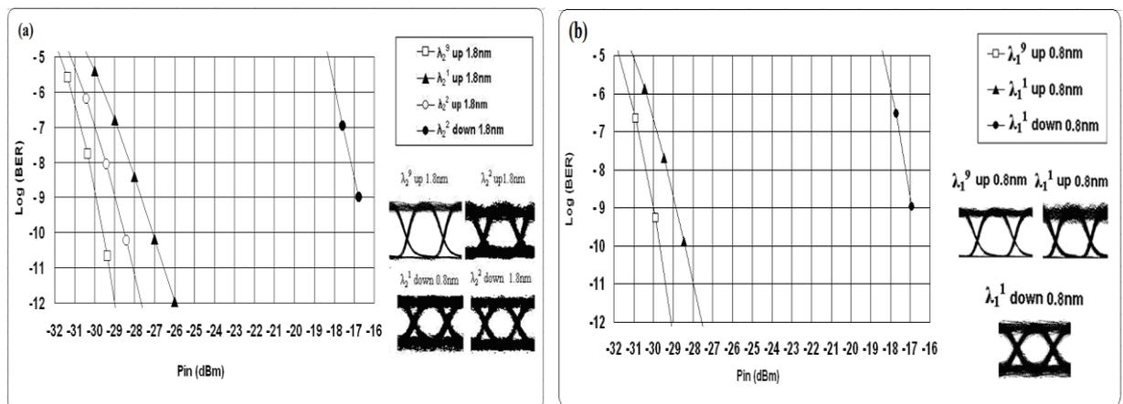
Figure 5-15 Measured BER for upstream and downstream transmission at (a) 0.8 nm (b) 1.8 nm
