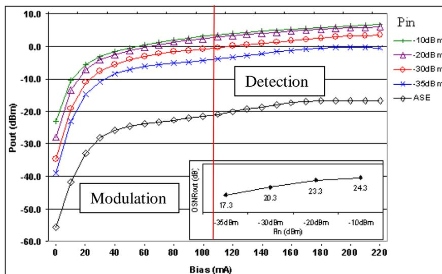
Figure 5-2 RSOA reflected signal and ASE noise power versus bias current
