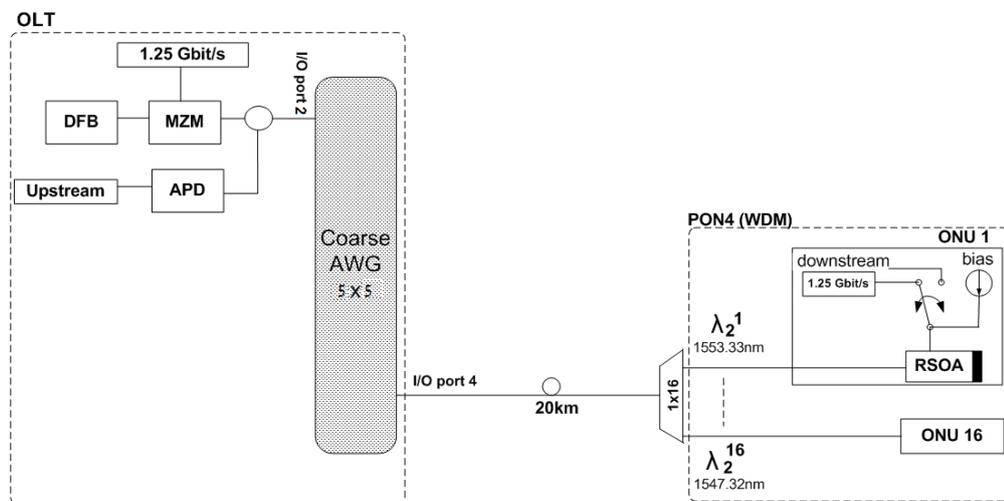
Figure 5-14 Simulation testbed utilising RSOA-based ONUs
