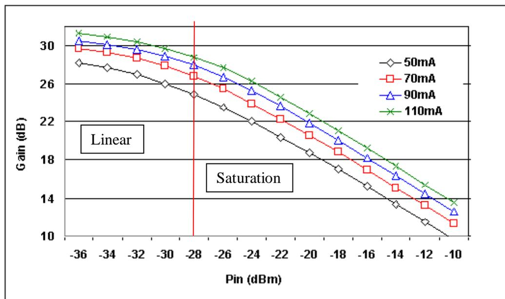
Figure 5-3 RSOA gain versus injected signal power
