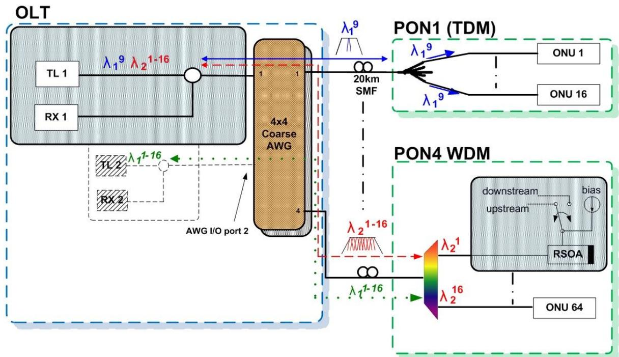
**Figure 5-1** An interoperable access network based on CWDM-routed reflective PONs
