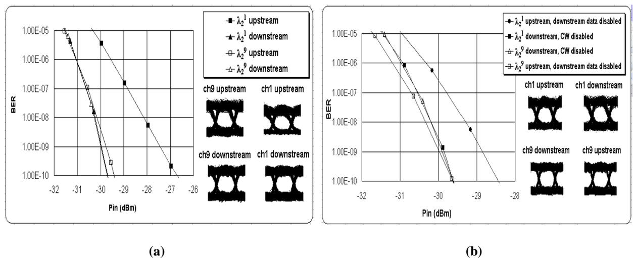
Figure 6-6 BER for (a) full-duplex bi-directional (b) half-duplex upstream and downstream transmissions
