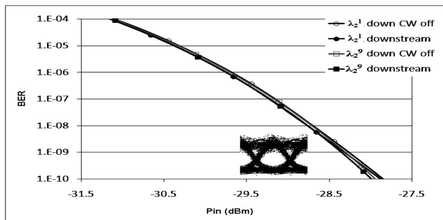
Figure 6-7 Measured BER for upstream and downstream transmission at 10 Gbit/s
