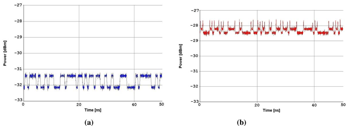
**Figure 6-5** Injected CW at RSOA optical input (a)  $\lambda_2^1=1553.33$  nm (b)  $\lambda_2^9=1550.12$  nm
