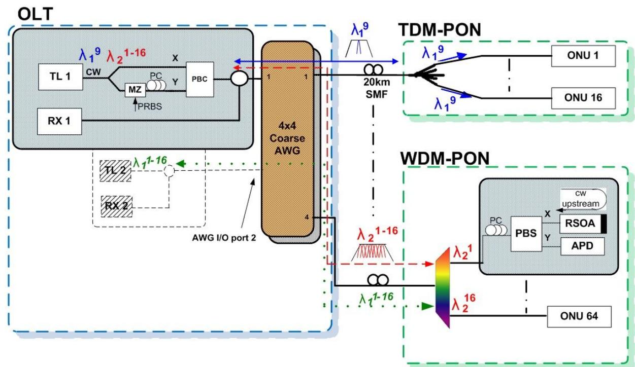
Figure 6-2 Full-duplex CWDM-routed reflective PONs network architecture
