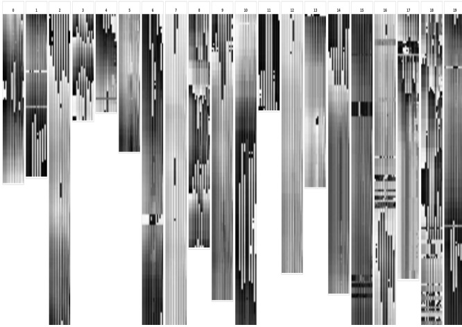
Fig. 2: The two dimension representation of x position from 20 videos with different length in robot view from walking action
