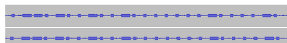
Fig. 1. Sequential key presses on the Kerui alarm arming fob, illustrating the lack of rolling codes.
