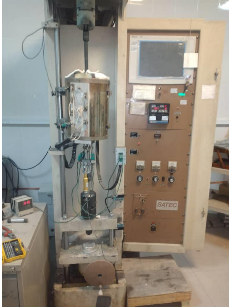
Figure 3-9. Test setup apparatus used for the creep testing
