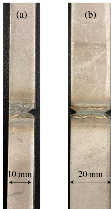
Figure 4-9. Notched samples prepared for cyclic tests: (a) single-edge, (b) double-sided V-shaped notch.
