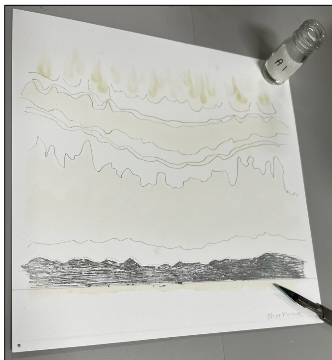
Figure 79: Outlining and extracting secondary metabolite segments from the preparatory TLC plate. The image below indicates a sample has been removed from the plate using a scalpel blade, revealing the underlying supporting aluminium sheet. The silica containing the isolated secondary product is weighed and stored in a small, labelled glass bottle. The procedure is repeated for each identified layer
