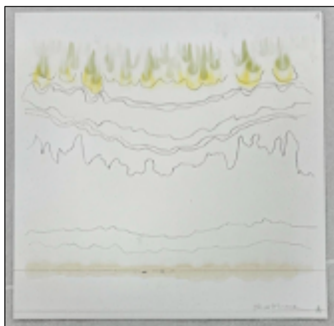
Figure 55: Preparatory TLC plate separating extracts obtained from O. parella . Variations in the line-front are common, reflecting imperfections in the silica layer varying resistance to the eluent as it rises upwards, depositing component compounds
