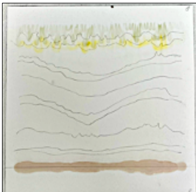
Figure 56: Preparatory TLC plate separating extracts obtained from R. siliquosa . Variations in the line-front is common, reflecting imperfections in the silica layer varying resistance to the eluent as it rises upwards, depositing component compounds
