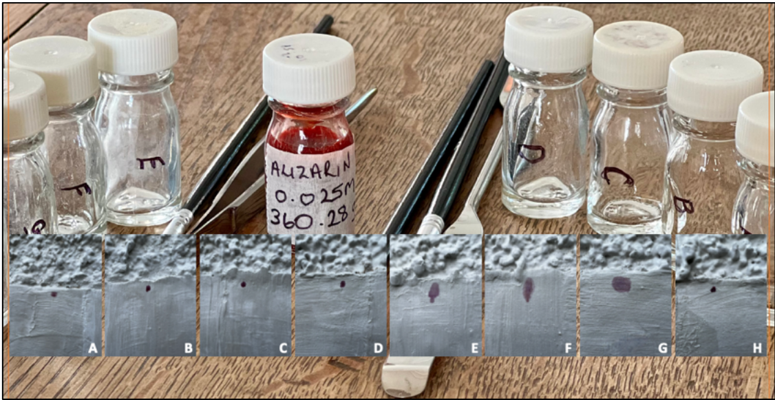
Figure 30: The impact of Alizarin Red dye onto sections A – H, applying 0.1 ml of Alizarin Red (0.025M). The dye readily penetrated the limewash through open pores. Reduced pore accessibility to the dye resulted in horizontal spread on the surface of the limewash observed on sections E, F, and G
