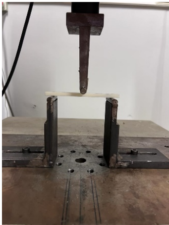
FIGURE 4: TESTED SPECIMEN AND THREE-POINT BENDING TEST SETUP
