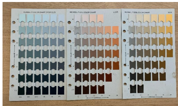
Figure 4.3 Example of Munsell soil colour charts used in this study. Pages from Macbeth Division, 1994.
