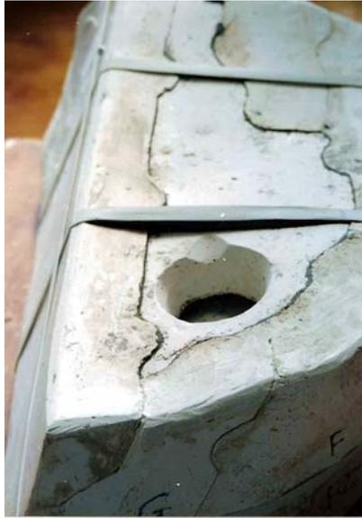
**FIG. 20. Mould, Detail of pouring hole and straps**
