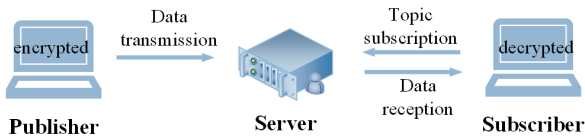
Fig. 19: Data sharing structure of the MQTT.
