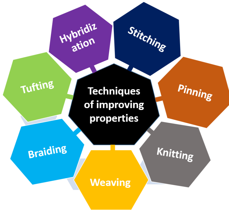
Fig. 12. Various potential techniques of enhancing properties of animal-based composites.
