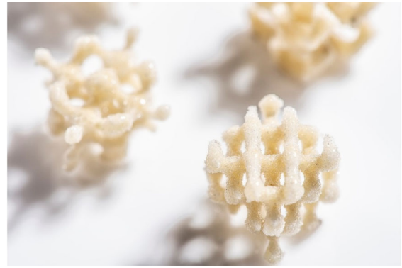
Fig. 1 Additively manufactured lattice structures of soda lime silica glass with laser powder bed fusion (Datsiou et al. 2021)
