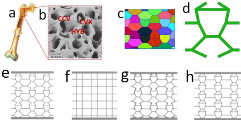
**Figure 3.** (a) Bone trabeculae, (b) trabecular bone closed cell plate-like structure, which was made up of (c) a Voronoi diagram that mimics trabecular bone, (d) a unit cell that was taken from the Voronoi diagram [5], (e) biomimetic, (f) square, (g) fillet and (h) repeated designs.
