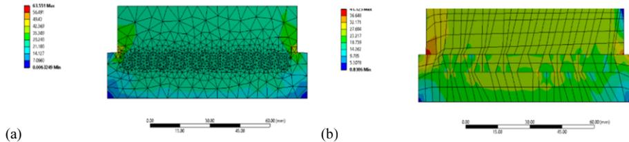
**Figure 4.** Stress distribution in (a) biomimetic and (b) triangular designs under tensile load.
