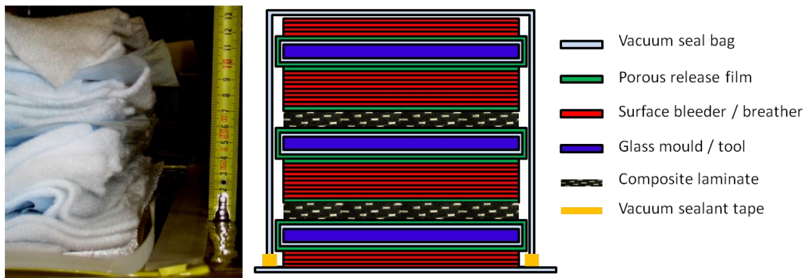
Figure 4.7: Bagging schedule for production of laminates A1 to A6 and L1-L3.
