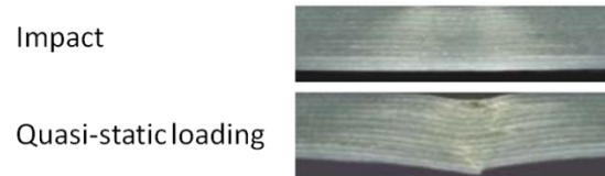
Figure 3.11: Damage extension seen in the direction of the fibres oriented to 0^\circ at the centre plate cross section (Rilo et al. (2006)).
