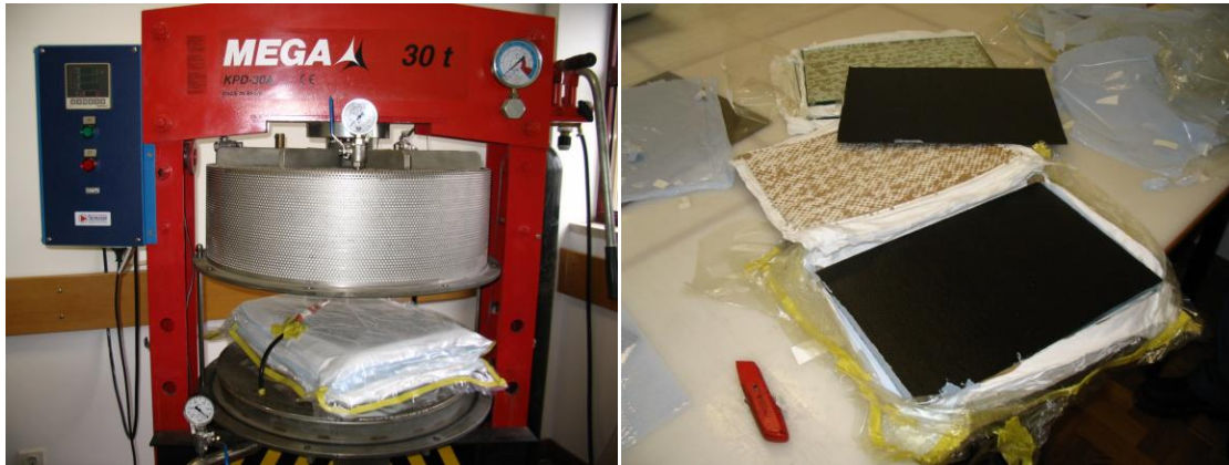
Figure 4.2: ISEL's autoclave with the bagging schedule inside (left) and raw plates obtained after the polymerization process (right).
