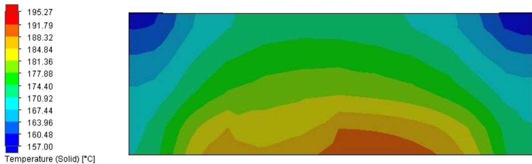
Figure 31. Temperature distribution in the middle plane of the window parallel to side b, CR:8.14 at 1500 rpm
