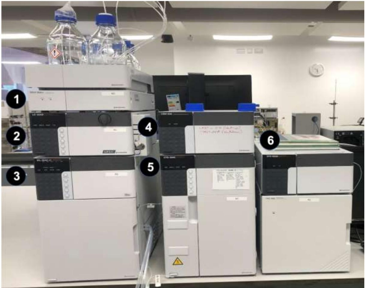
**Figure 2.3: Shimadzu Prominence HPLC machine with various component units. Degassing Unit (DGU-20A5R) (1), Liquid Chromatograph (LC-20AD) (2), Autosampler (SIL-20AC HT) (3), Communications BUS module (CBM-20A) (4), Column oven (CTO-20AC) (5) and a diode array detector (SPD-M20A) (6).**
