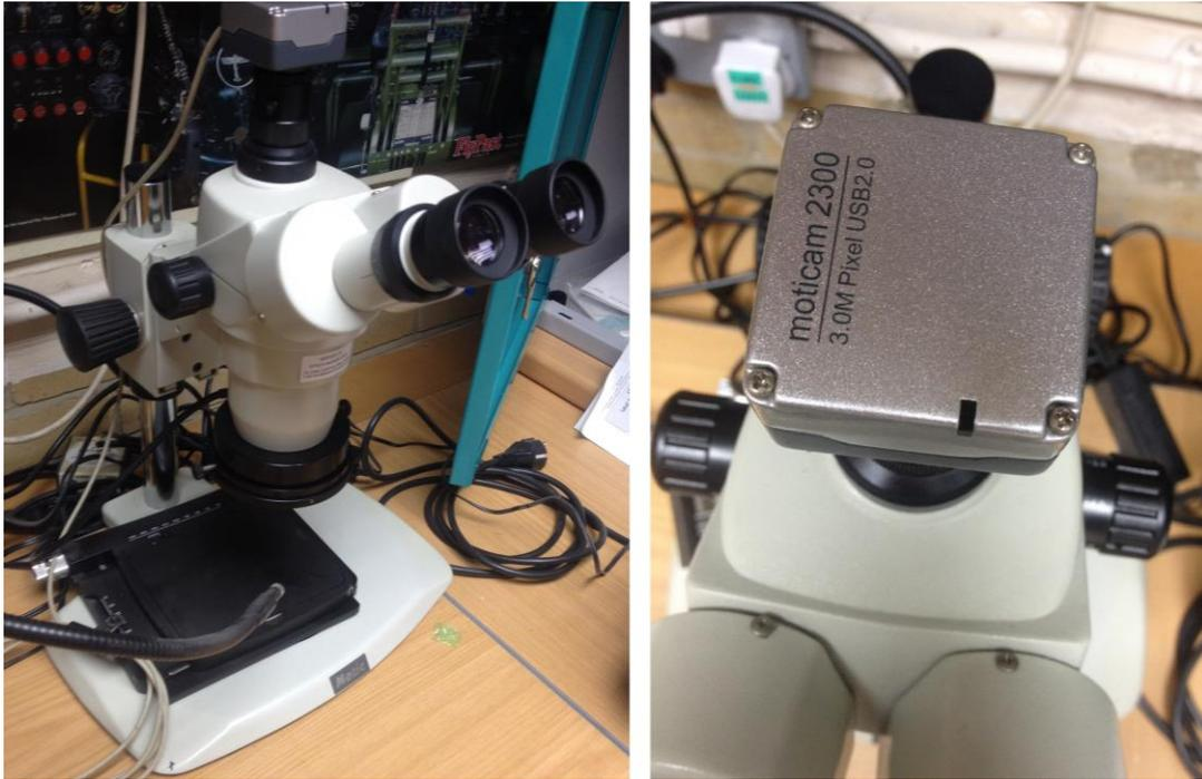
**Figure 6.19 Motic microscope system and its built-in Moticam camera.**
