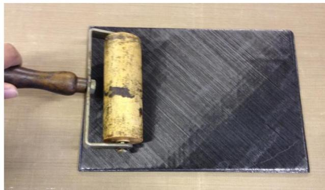
(b) A layered laminates is rolled by a hand roller.
