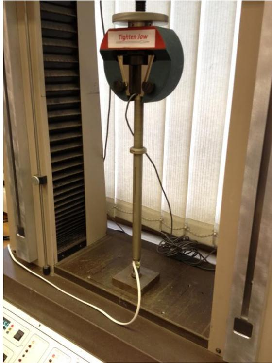
**Figure 5.6 Calibration of the impactor with strain gauge bonded.**
