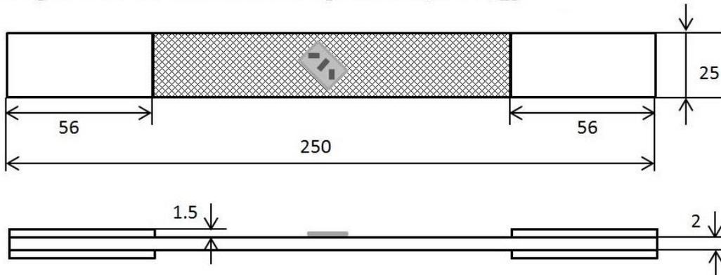
**Figure 4.11 Schematic illustration of the in-plane shear modulus test specimen.**
