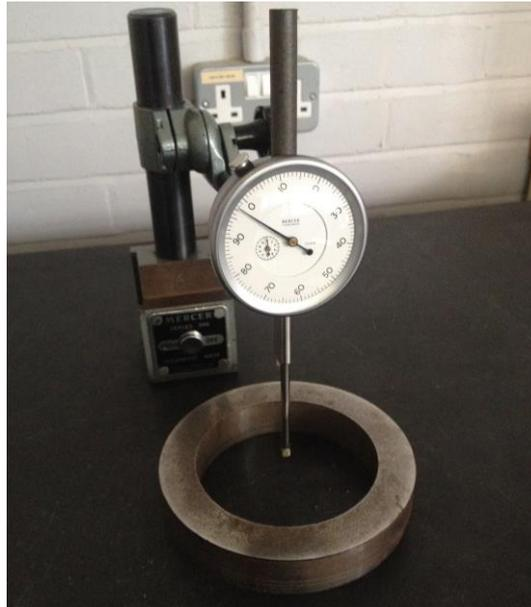
**Figure 6.3** Depth dial gauge to measure dent depth.
