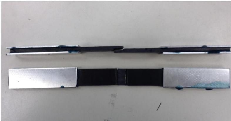
**Figure 4.16 Specimens failed under the interlaminar shear stress.**
