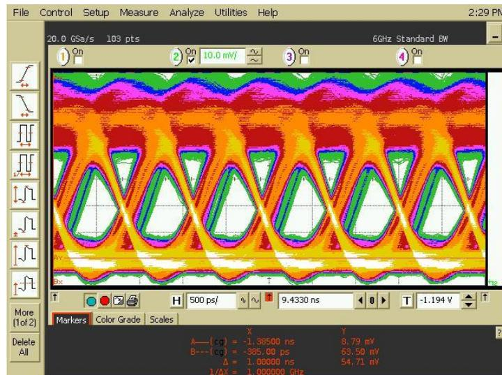
Figure 7-4 Extinction ratio of the experimental RSOA transmitted signal
