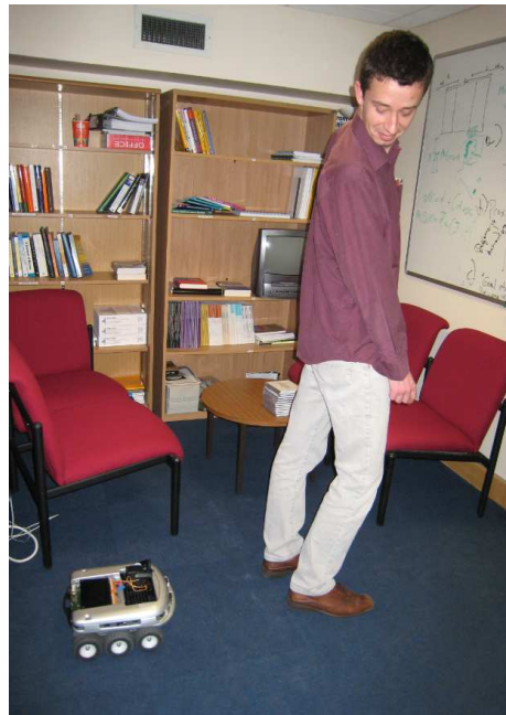
Figure 4: Setup using a Koala robot learning to follow the experimenter.
