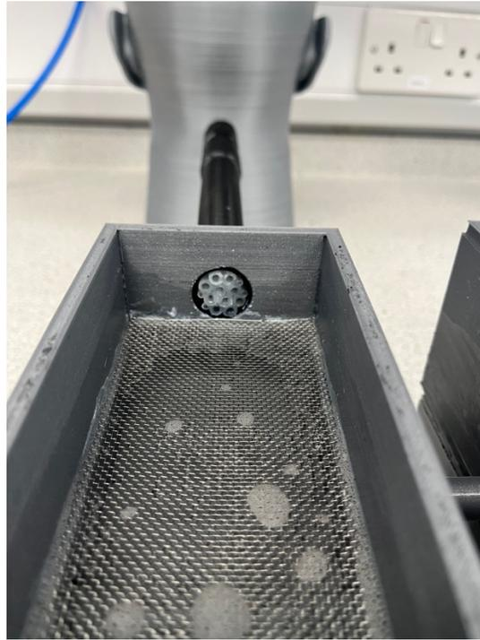
**Figure 18.** Photographs of the perforated stainless-steel sheet seated in the system reservoir a) 10 mm below the lower aspect of the exit port (entry port not visual) during pilot tests with the polylactic acid prototype and b) at a flush level with the lower aspect of the exit port representing the finalised position in the solvent-welded, polyethylene terephthalate glycol prototype.
