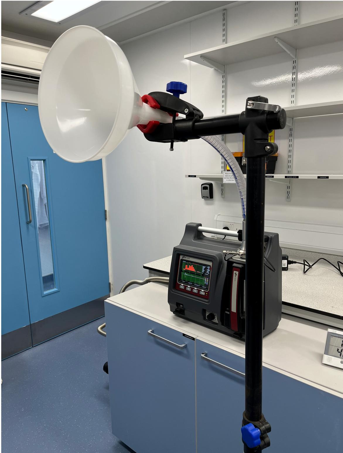
**Figure 17.** Photograph of equipment set-up for the human cough experiments. Positioned approximately 50 mm from the funnel opening, participants were asked to produce a single volitional cough into the funnel, considered to be a semi-confined environment. The ELPI+ machine was connected directly to the funnel via a flexible polyurethane hose.
