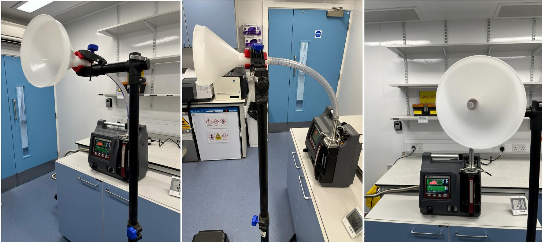
**Figure 185.** Images showing the equipment set-up during the characterisation of a human cough experiment. Positioned approximately 50 mm from the funnel opening, participants were asked to produce a single volitional cough into the funnel, considered to be a semi-confined environment. The ELPI+ machine was connected directly to the funnel via a flexible polyurethane hose.
