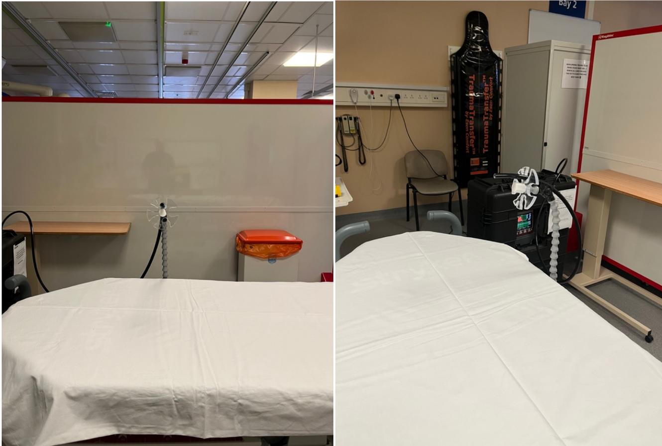
**Figure 29.** Images of the trial set-up for work package two (emergency department setting). The black sampling tube was held in position by a tube holder which slides into place beneath the trolley mattress. The ELPI+ equipment, housed within a Peli case for protection and ease of movement, can be seen in the background of the image (right). The sampling tube would be situated approximately 10 cm from a patient's mouth opening.
