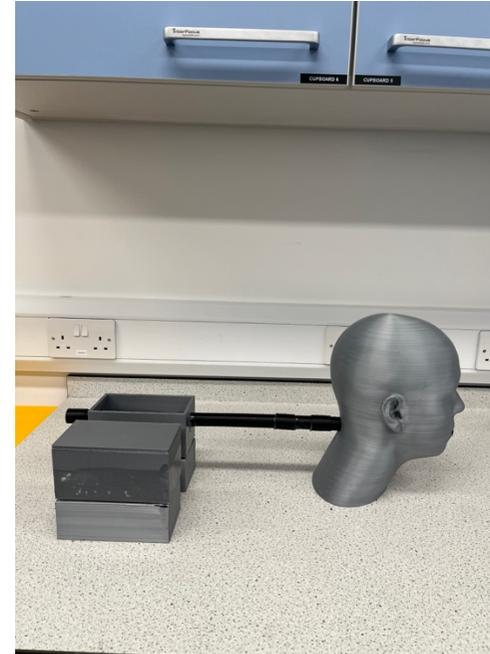
**Figure 170.** Photographs of the NACS design, highlighting anthropomorphic characteristics pertinent to aerosol generation. 1mm perforated stainless-steel mesh and a network of silicone tubing can be seen within the system reservoir exit port. These features represent mechanisms of fluid film burst and vibration between structures in close proximity, respectively.
