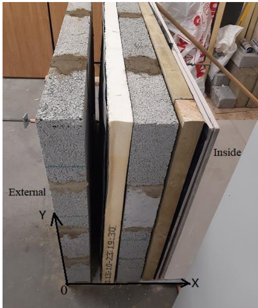
(a). Layered wall construction
