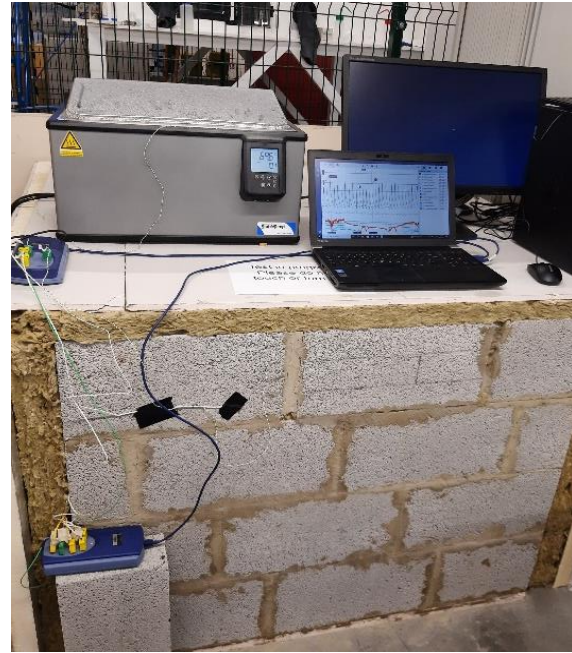
(b). Calibration in boiling water in thermo-bath
