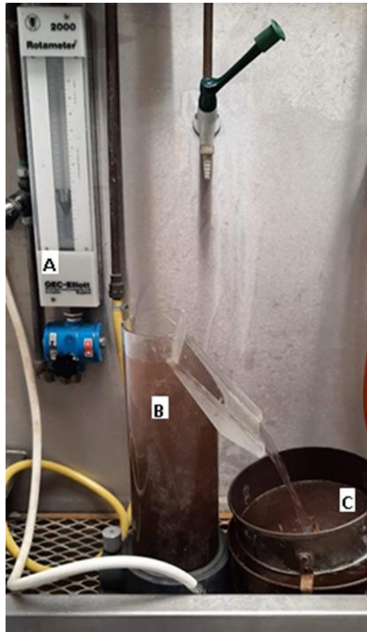
Figure 2.1: Heterodera schachtii cyst nematode collection using Wye washer. Soil samples were placed in the Wye washer with a small amount of water (B), to separate cyst nematodes from larger soil debris. The Rotameter (A) was then set to 7.5 L/ min. The outflow ran through two sieves (850 \mu m and 250 \mu m mesh). The cyst nematodes were collected in the 250 \mu m sieve (C), filtrate was then processed as described in Section 2.1.1.
