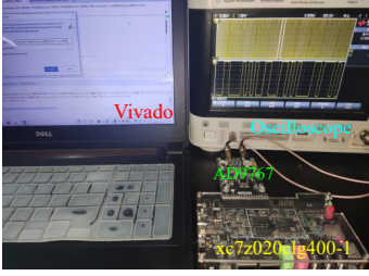
Fig. 18: PRNG implementation based on an FPGA hardware platform.
