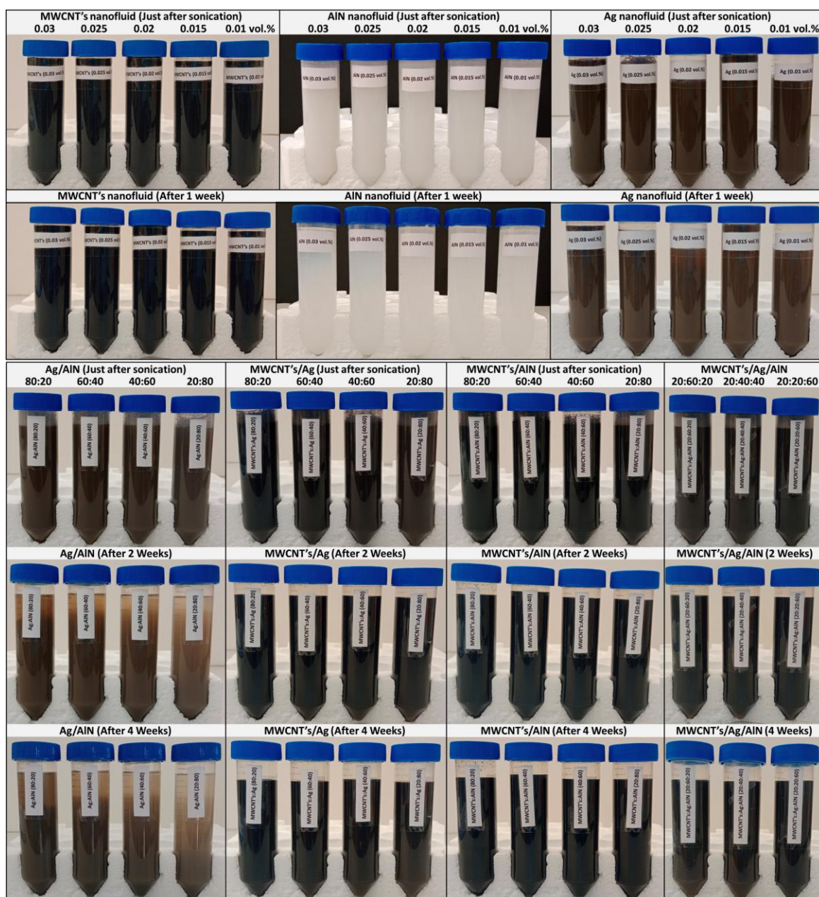
Figure 6.9. Stability comparison of hybrid and tri-hybrid nanofluid samples.
