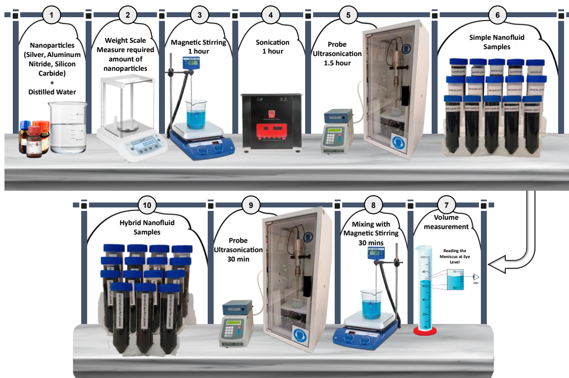
Figure 6.2. Schematic diagram of nanofluid preparation steps for simple and hybrid samples.
