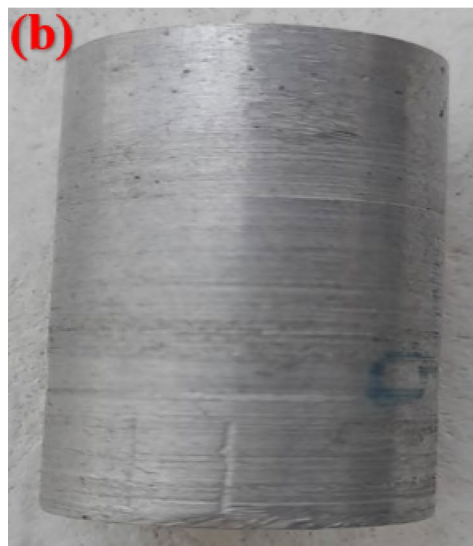
Fig. 2. (a) WEDM machine setup and (b) WEDM workpiece samples.
