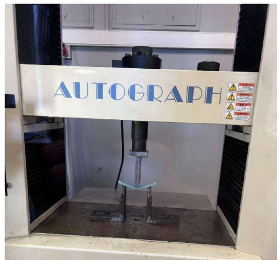
Figure 3. Three-point bending test setup.
