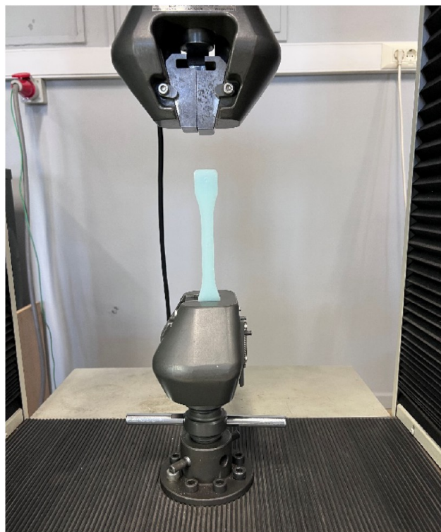
Figure 2. Tensile testing sample and test setup.
