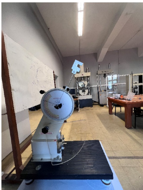
Figure 4. Charpy impact test setup.
