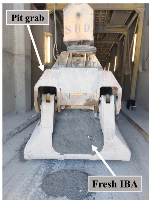
Fig. 1. Pit grab filled with fine, fresh IBA during sample collection at the waste-to-energy (WtE) plant.
