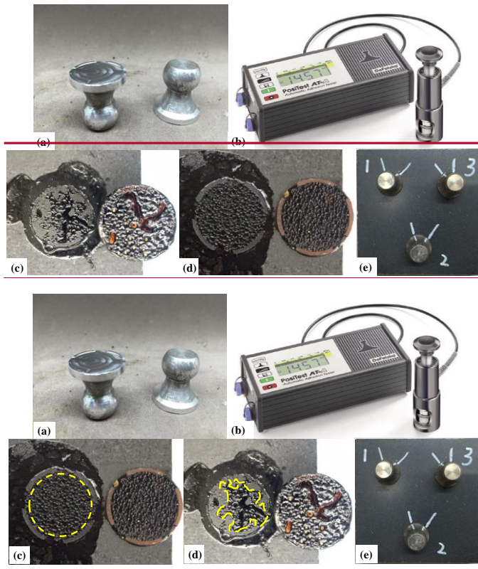
Figure 1 (a) Stubs and (b) Positest AT-A apparatus and (c) cohesive failure and (d) adhesive failure and (e) samples with marks
