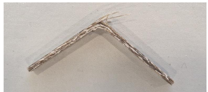
Figure 22 NF sample after impact test
