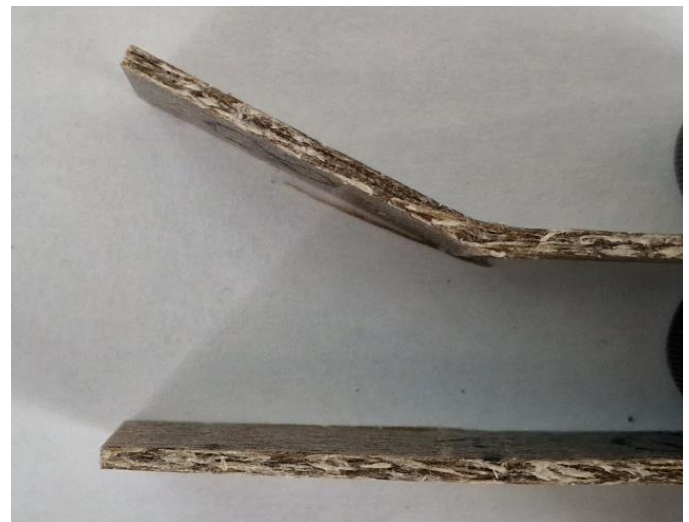
Figure 18 NF samples after flexural test
