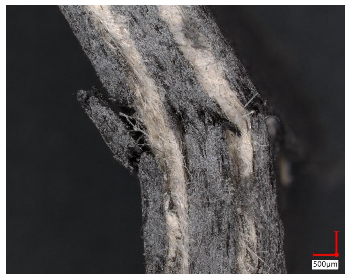
Figure 23 Magnified view of impact failure of layup 5
