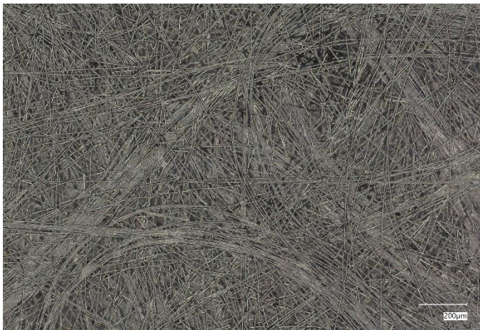
Figure 4 Magnified view of rCF after manufacture
