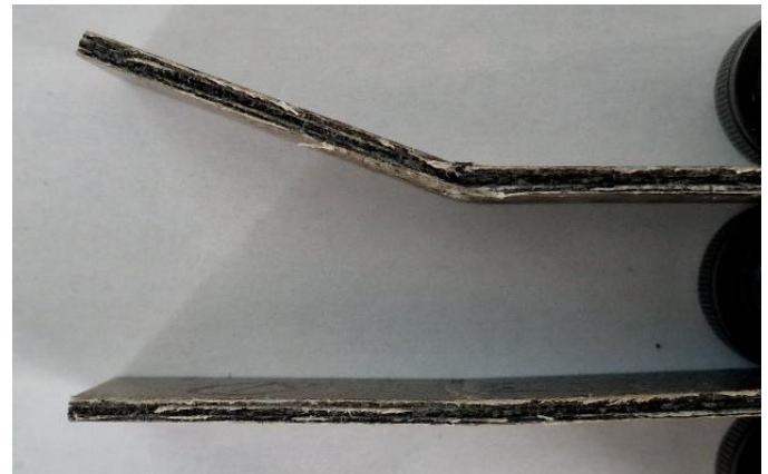
Figure 17 Hybrid samples after flexural test
