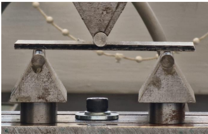
Figure 7 Flexural test setup
