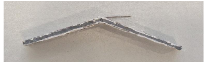
Figure 21 Hybrid Sample after impact test
