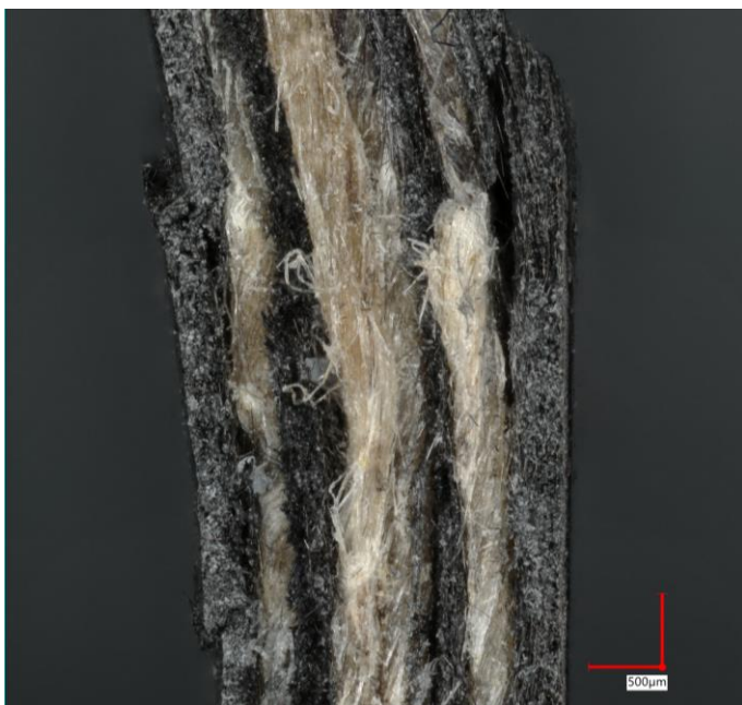
Figure 15 Magnified view of the flexural failure of layup 6
