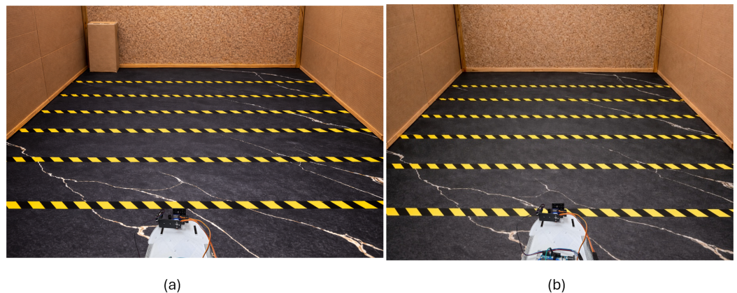
Figure 5. Experimental environment used for evaluating the proposed LiDAR scanning system. The experiments were conducted in a small indoor test arena ( 1.6 \text{ m} \times 2.0 \text{ m} ) with distance markers placed along the floor to provide reference intervals. The mobile robot equipped with a servo-actuated LiDAR scanner was positioned at the starting location, while a rectangular cardboard obstacle was placed within the LiDAR's field of view. (a) Experimental setup with an obstacle present. (b) Baseline environment without an obstacle.
