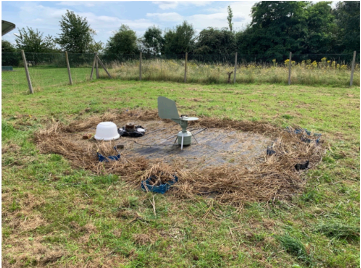
Figure 5.3: Infected oilseed rape stubble from the previous growing season placed around the Burkard spore sampler set-up at Bayfordbury, Hertfordshire.
