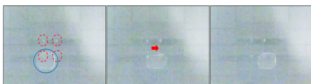
Figure 9. Droplet movement across one middle electrode, from electrode 6 to electrode 11. There are four middle electrodes with the vias positioned at the top left corner of each electrode. In the first image, the droplet is indicated in the blue circle while the four vias are indicated inside the dashed red circles. Initially, the droplet was positioned on electrode 6 (the bottom left electrode of the four middle electrodes). The second image shows the elongation of the droplet during its transportation to the next electrode as electrode 11 was activated. The red arrow indicates the direction of droplet movement. The third image shows the droplet in its final position, on electrode 11. (Photograph courtesy of E. Nadia. Copyright 2025).
