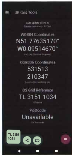
Figure 2. UK Grid Tools screenshot showing available formats and the copied value in the bottom left corner. The number of digits can be changed in Settings.
