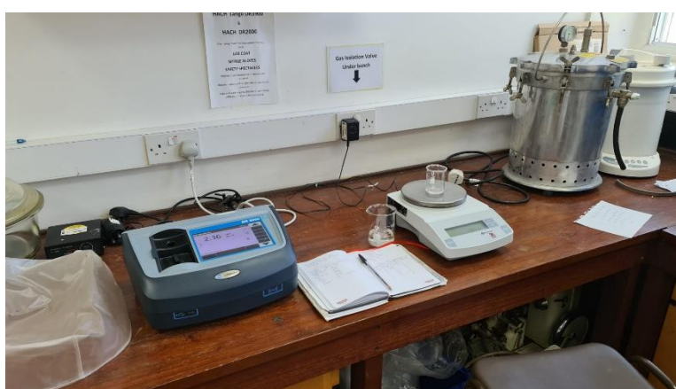
Figure 4. 4: Left: The laboratory set up for the HACH machine cuvettes for ammonia, phosphate and nitrates. Right: The HACH machine and balance machine to calibrate the pipettes.
