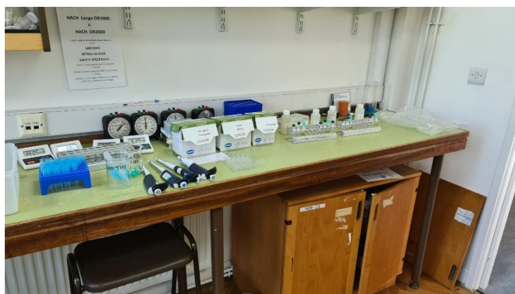
Figure 4. 4: Left: The laboratory set up for the HACH machine cuvettes for ammonia, phosphate and nitrates. Right: The HACH machine and balance machine to calibrate the pipettes.
